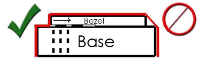
Without the proper spacing between the top bezel and the base piece the plastic will have a tendency to pull right over the base corner instead of pulling down around the bezel then around the base as it should. Placing thin 1/16th thick spacers underneath the bezel and drilling holes through the base will allow for the suction to get through, but not suck the plastic under the bezel.
