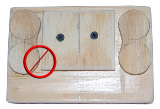
As you can see, the space between these two components would not be enough for the plastic to sink into, on top of the fact there is no place for the suction to even get to the component.
